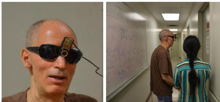
**Fig. 15.** Example of a prototype system includes a Logitech web camera with auto focus on sunglasses.
