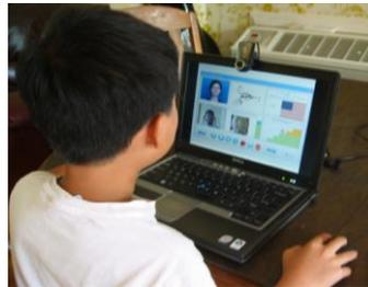
**Figure 2:** The basic hardware configuration of the proposed interactive intelligent tutoring system, which includes a computer (desktop or laptop), a web camera with auto focus (face to the user), and a microphone.
