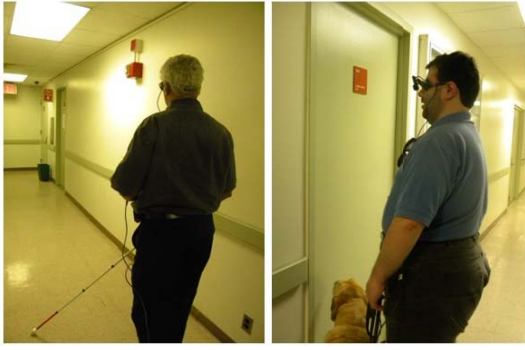
Fig. 1. Testing our prototype system with a wearable camera for blind navigation.
