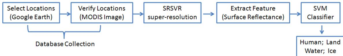
**Figure 2:** Flowchart to evaluate the feasibility of human activities detections using the SRSVR super-resolution algorithm.
