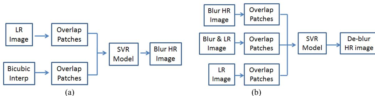
**Figure 4:** Flowchart of the SRSVR super-resolution algorithm in two steps: (a) up-sampling and (b) de-blurring.
