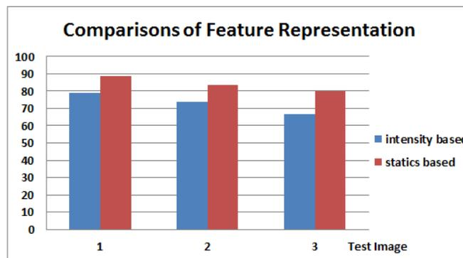
**Figure 7:** Comparison between the statistics based feature representation with the intensity based feature representation at the super-resolution scale of 4.
